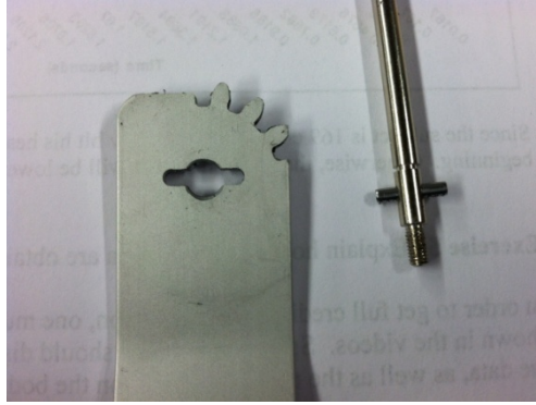
Figure 67: Hinged Arm with Mating Pinned Transmission Shaft
