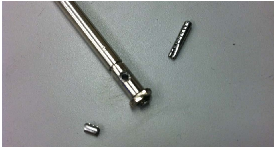
Figure 81: Pin Failure due to Shear
