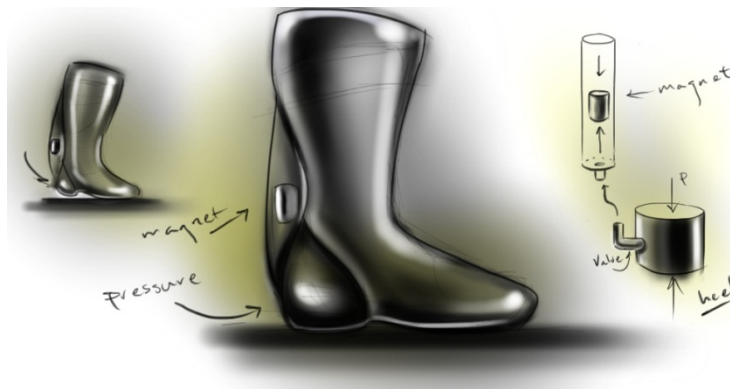
Figure 25: Concept Design of Linear Actuator Electromagnetic Boot
