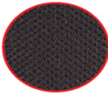
Figure 37: Texture Sample of Neoprene/Polystyrene Blended Material
