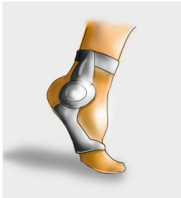
Figure 24: Concept Design of Electromagnetic Ankle Brace Generator
