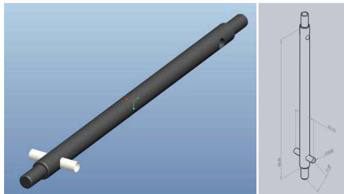
Figure 61: SolidWorks Solid Model & Wireframe Views of the Shaft and Pin Assembly
